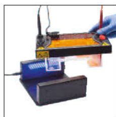
blue light source features a sliding panel to accommodate both MINI and MIDI units
