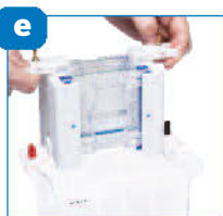
Transfer to tank and fill with buffer
