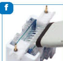
Load samples using Loading Guides and run
