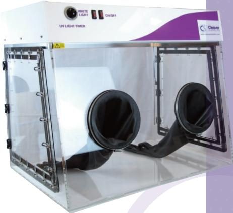
The Cleaver Scientific Combi Box combines the benefit of UV sterilisation with the fully sealed and enclosed area of a glove box. Four 15W UV-C bulbs may be timer controlled for up to 30 minutes, or indefinitely, to decontaminate equipment and the work surface
