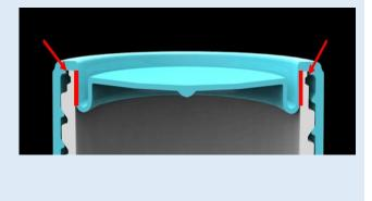
Increased the thickness of conical bottom in order to improve the maximum centrifugal limit.
