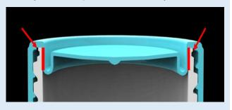
Increased the thickness of conical bottom in order to improve the maximum centrifugal limit.
